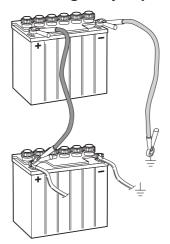
Connect each end of the red cable to the POSITIVE pole (+) on each battery, exercise care not to short circuit any of the ends against the chassis.
